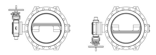
Horizontal installation position is recommended for all butterfly valves with the gearbox facing up or down (see the picture above).
