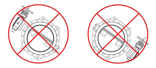
Vertical or inclined installation position is forbidden (see the picture above).
