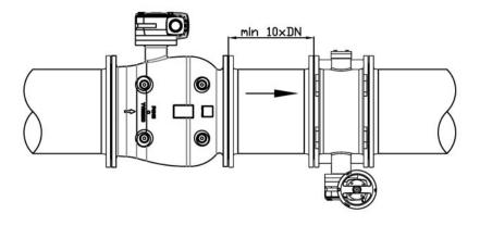
When installing a butterfly valve downstream of a control valve or a plunger valve, make sure that there is enough space between them (minimum  $10 \times DN$ ).
