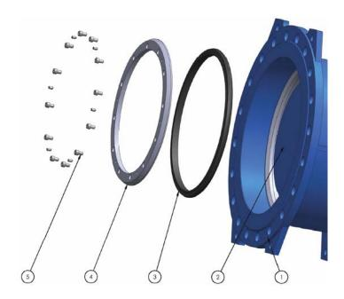
Due to the double-eccentric bearing, the profile seal can be replaced without disassembly of the disc and all safety precautions need to be taken.
